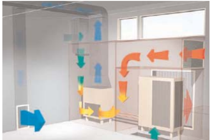
DV delivers conditioned 100% outside air.
