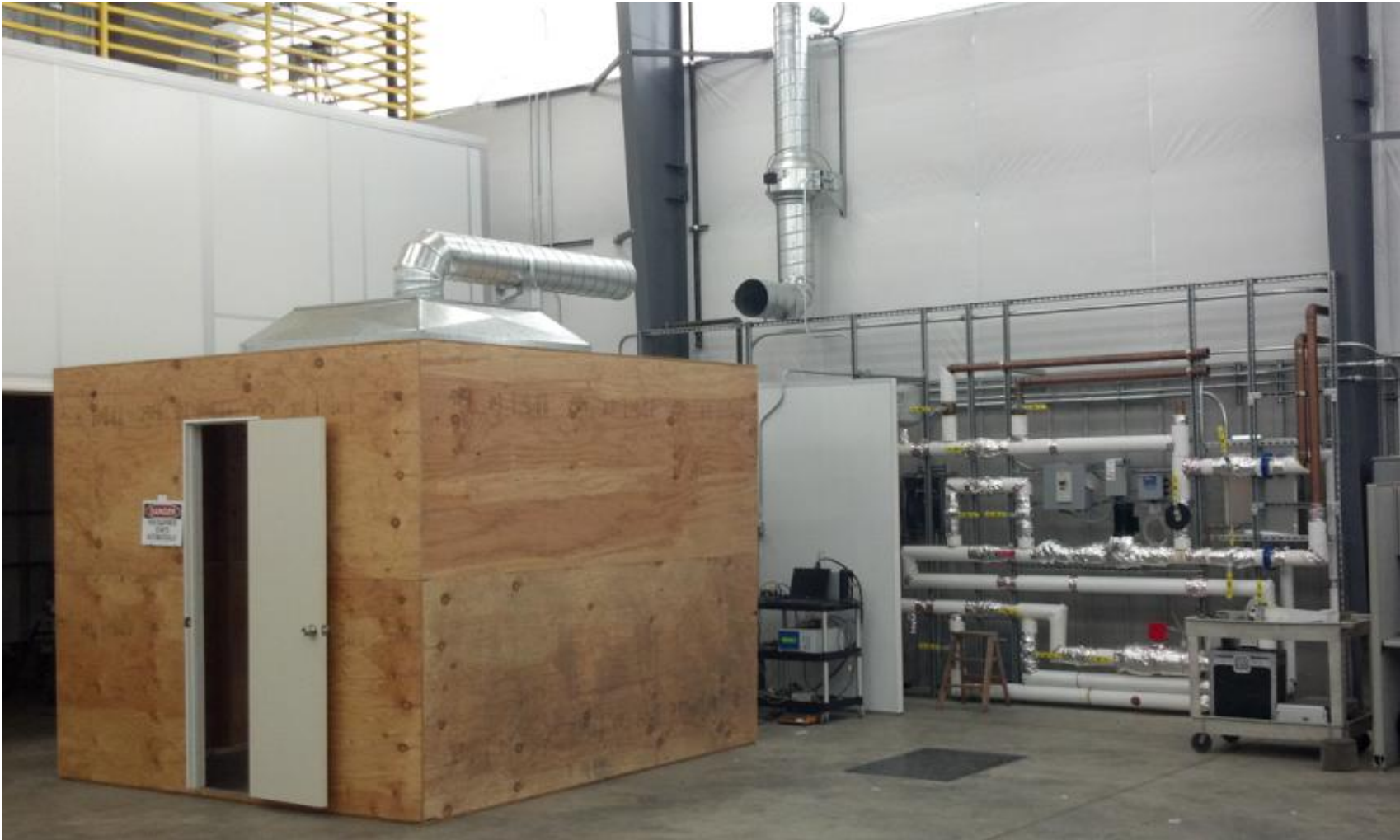
FIGURE 2. BOILER TEST APPARATUS
