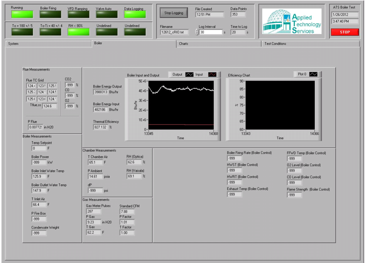
FIGURE 15. LABVIEW BOILER SCREEN
