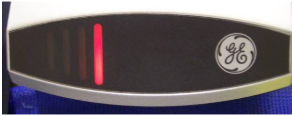
Figure 6: DR Module and HPWH Display in Level 3 / Critical Mode
