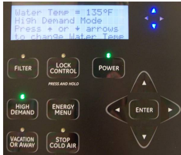
Figure 3: DR Module and HPWH Display in Normal or “Low” Mode
