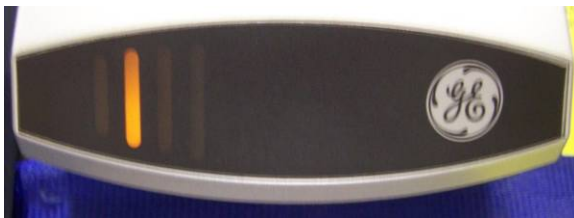
Yellow light, second from left indicates Level 1 response
