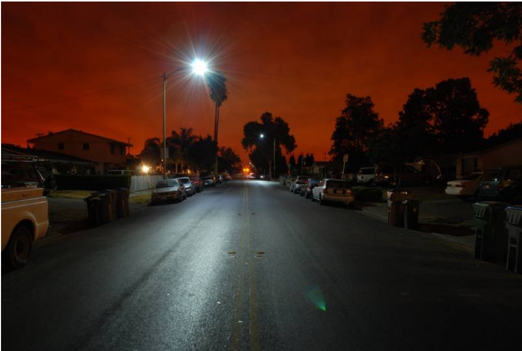
Figure 24: Street Level Shot, LED 50%
