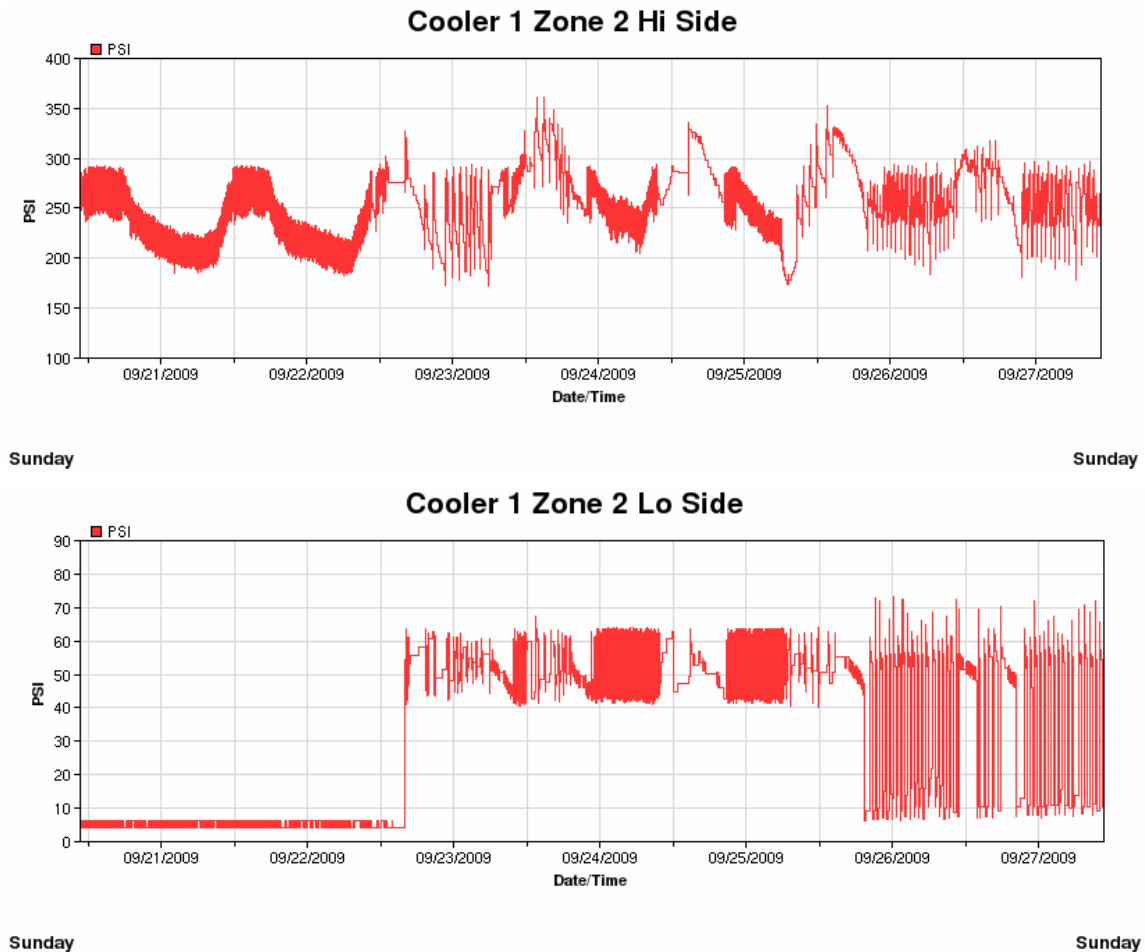
FIGURE 19 C1Z2 PRE-MAINTENANCE DISCHARGE & SUCTION PRESSURES
