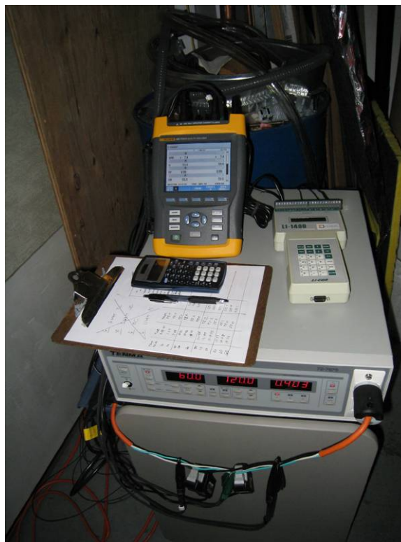
FIGURE 4. MONITORING TEST EQUIPMENT - REGULATED POWER SUPPLY, POWER QUALITY ANALYZER AND LIGHT LOGGING SYSTEM
