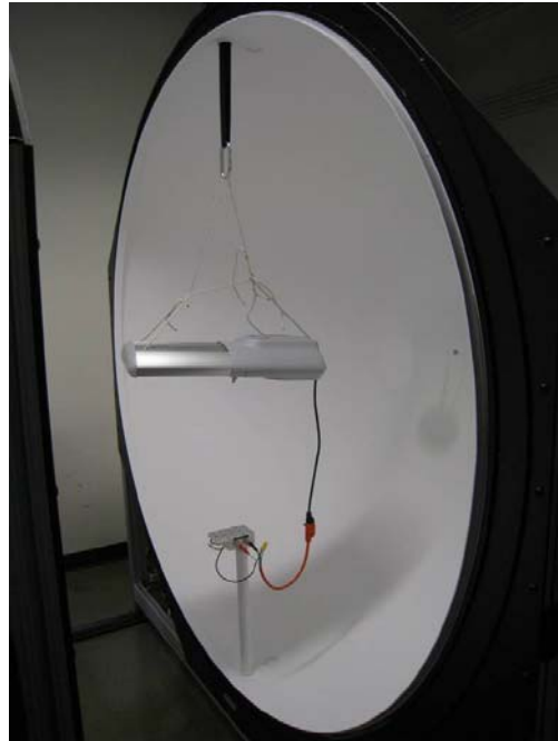
FIGURE 1. LUMINAIRE SETUP IN INTEGRATING SPHERE
