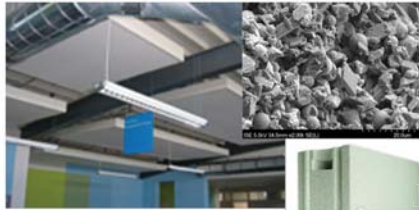
Phase change material to increase thermal storage
