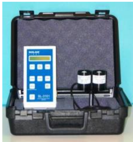
Figure 4: S/P Light Meter (Solar Light Company).
