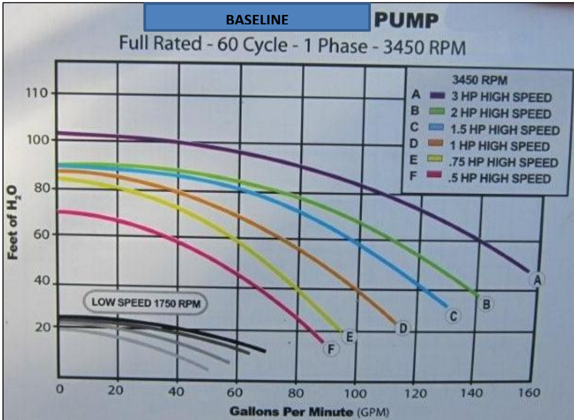
Figure 12: Baseline Pump Curve Chart
