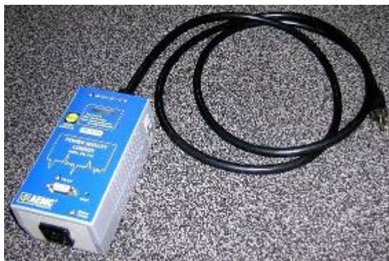
FIGURE 16. POWER QUALITY LOGGER
