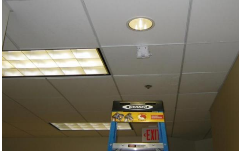
FIGURE 21. CORRIDOR OCCUPANCY SENSOR LOGGER MOUNTED ON CEILING TILE T-BEAMS. (TWO OCCUPANCY LOGGERS WERE USED TO MONITOR ACTIVITY IN THE CORRIDOR TEST AREA, PICTURED IN FIGURE 22.)
