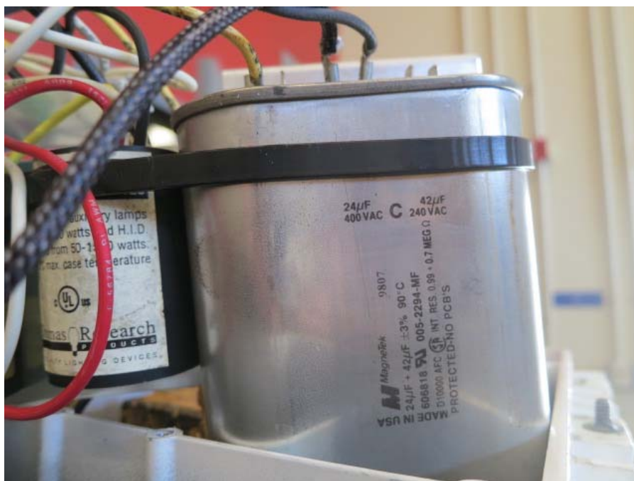
FIGURE 7: MULTI-TAP CAPACITOR – CORRECTLY WIRED FOR 24 µF DURING TESTING
