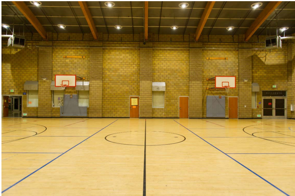
FIGURE 10: INSTALLED LED FIXTURE LIGHT LEVEL AND COLOR UNIFORMITY
