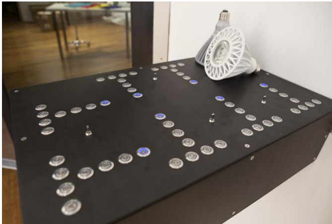
FIGURE 5. CONTROL PANEL FOR LED REPLACEMENT LAMPS IN LUX
