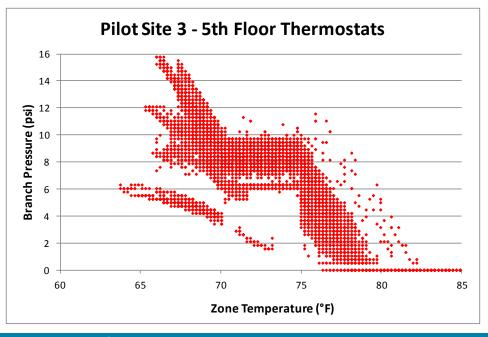
Figure 23: Pilot Site 3 - 5<sup>th</sup> floor Zone Temperature versus Branch Pressure
