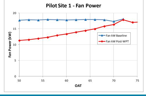
Figure 8: Pilot Site 1– Fan Power
