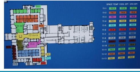
Figure 5: Pilot Site 1 - Thermostat Deadband Setpoints
