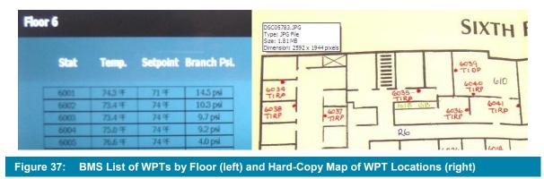
The figure above shows what we consider to be a poor display of WPT information because the thermostat locations are not shown graphically on the BMS screen.
