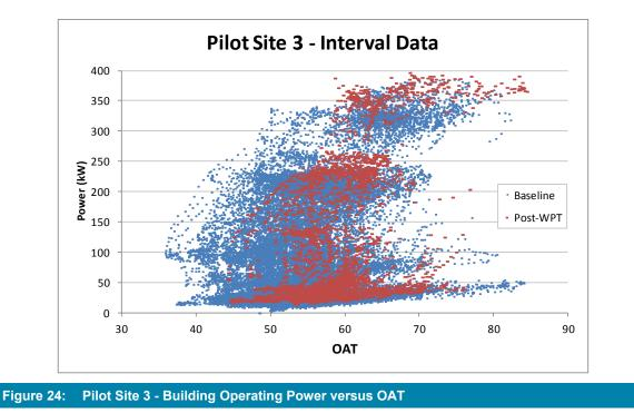
The figure above shows all hours of the building operation. Three clusters of data are visible: the top cluster represents operation when the chiller is on, the middle cluster represents non-chiller building operation, and the lowest cluster represents overnight operation.
