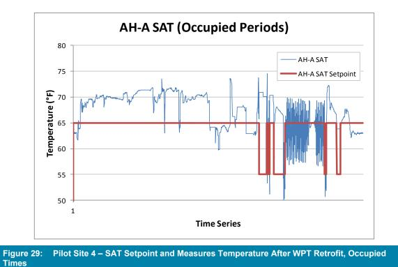
Finally, when we compare the observed supply air temperatures relative to outside air temperatures from before and after the WPT retrofit, we do not observe any significant difference. See the following figure.
