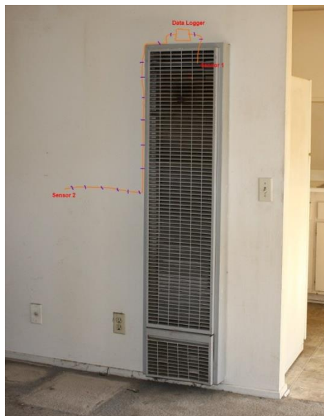
Wall furnace temperature measurements. Sensor 1 measures the hot supply air and sensor 2 measures the conditioned space air.
