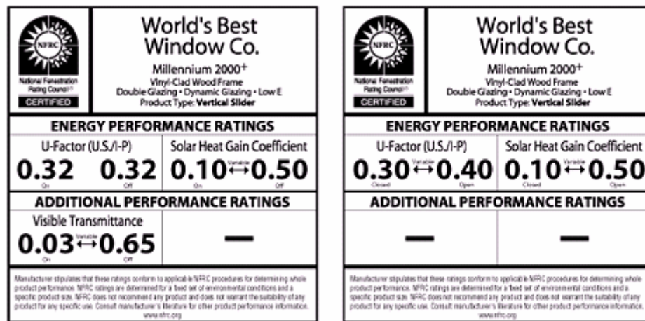
FIGURE 22. NFRC LABEL FOR DYNAMIC WINDOW GLAZING.
