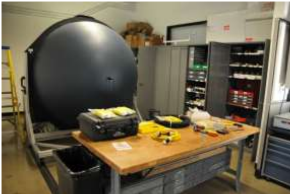
FIGURE 8. TECHNOLOGY TEST CENTERS' 2-METER SPHERE-SPECTRORADIOMETER LABORATORY (2MSSL)
