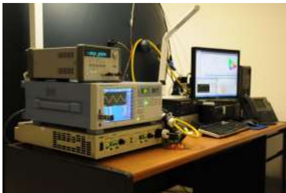
FIGURE 11. YOKOGAWA WT1800 PRECISION POWER ANALYZER (BLUE SCREEN IN MIDDLE), ELGAR CW1251P (BOTTOM), AND AGILENT E3634A (TOP)
