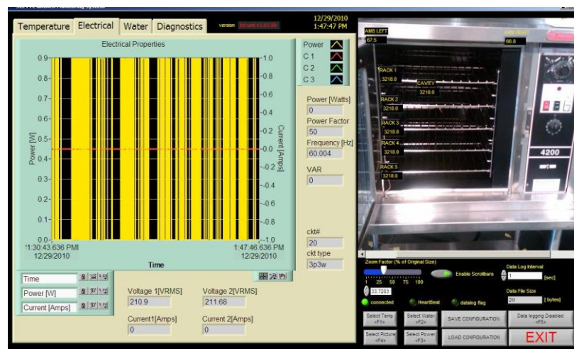
FIGURE 2. DAS INTERFACE WITH NATIONAL INSTRUMENTS LABVIEW
