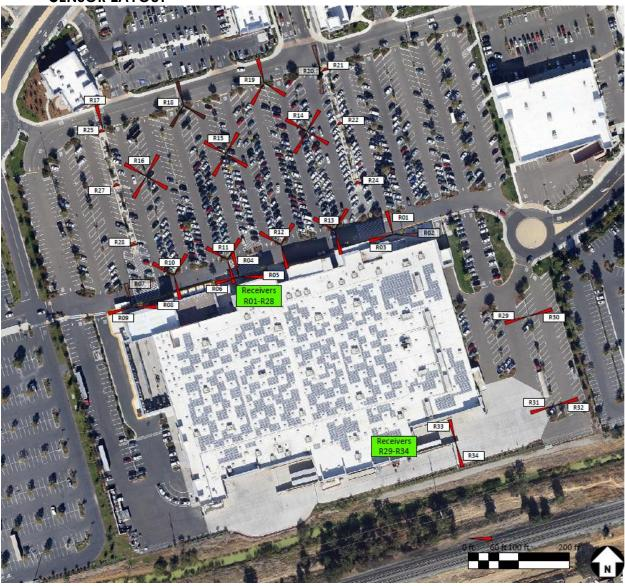
FIGURE 28: SENSOR LAYOUT AT THE BIG BOX STORE HOST SITE IN NORTHERN CALIFORNIA. R01–R34 REPRESENT THE LOCATIONS OF SENSORS AND RECEIVERS USED AT THIS SITE. THE RED TRIANGLES EXTENDING FROM THE RECEIVER LOCATIONS REPRESENT INDIVIDUAL SENSORS AND THEIR ORIENTATIONS.
