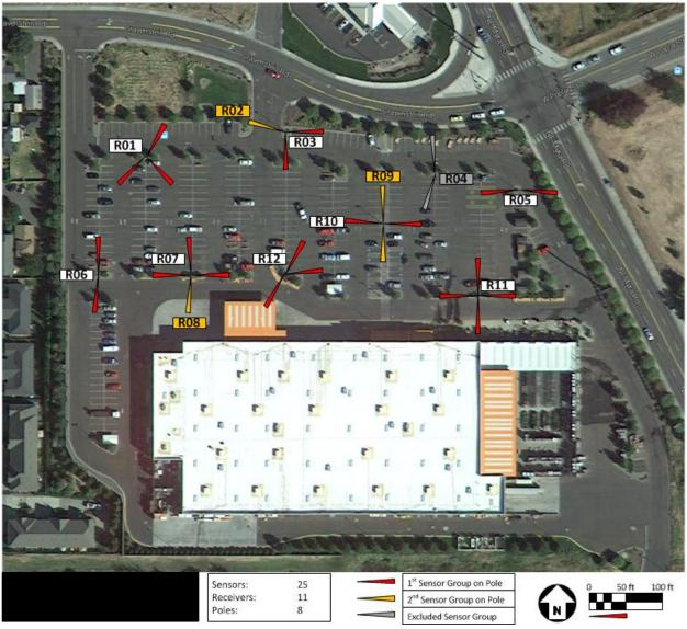
FIGURE 16: SENSOR LAYOUT AT BUILDING SUPPLY FRANCHISE HOST SITE.
