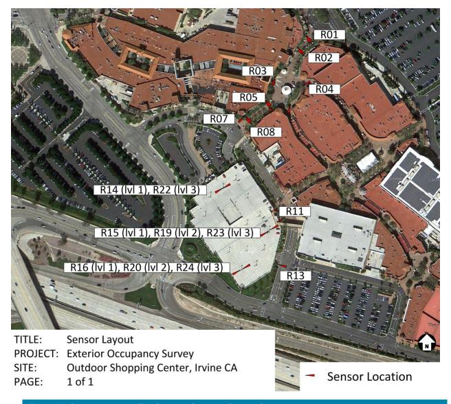
FIGURE 33: SENSOR LAYOUT AT THE OUTDOOR SHOPPING CENTER. SENSORS WERE PLACED THROUGHOUT THE PARKING STRUCTURE, ALONG THE WALKWAY BETWEEN STOREFRONTS AND ALONG THE ROADWAY. **R01–R24** INDICATE THE LOCATIONS OF THE RECEIVERS WHILE THE INDIVIDUAL SENSORS AND THEIR ORIENTATION ARE REPRESENTED BY RED TRIANGLES.
