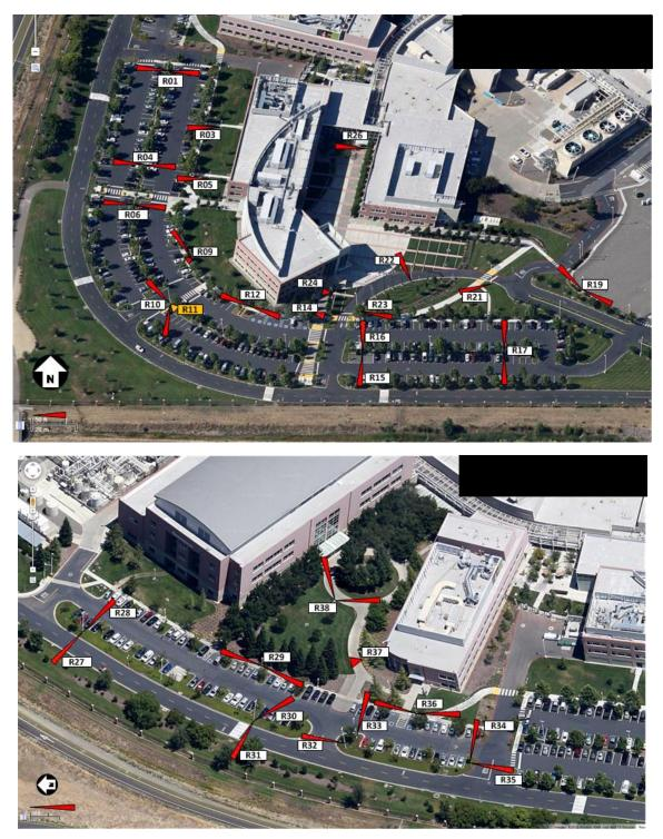
FIGURE 25: SENSOR LAYOUTS FOR OFFICE CAMPUS HOST SITE: AREA 1 (TOP) AND AREA 2 (BOTTOM).
