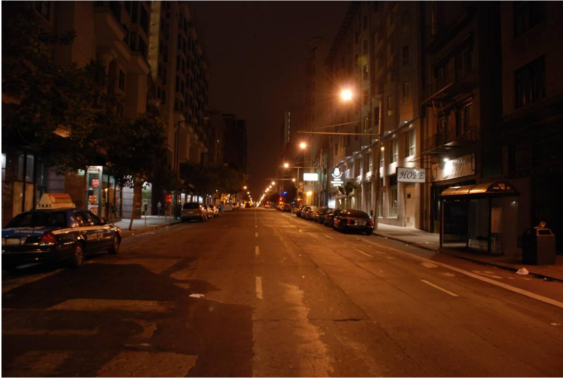
Figure 23: Street Level Shot of 200W HPS, Turk Street
