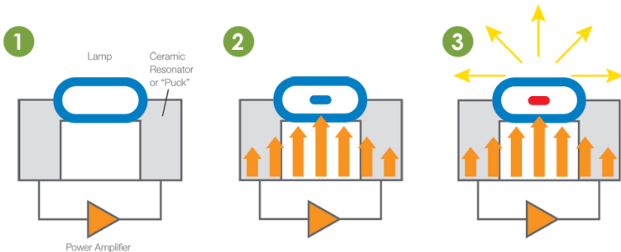
FIGURE 2. DIAGRAM OF HOW LIGHT EMITTING PLASMA WORKS (IMAGE SOURCE: LUXIM)
