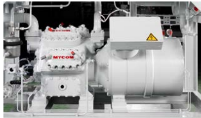
Semi Hermetic Compressor – No shaft seal
