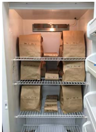
Incubator at 35°C and 52±1% RH
